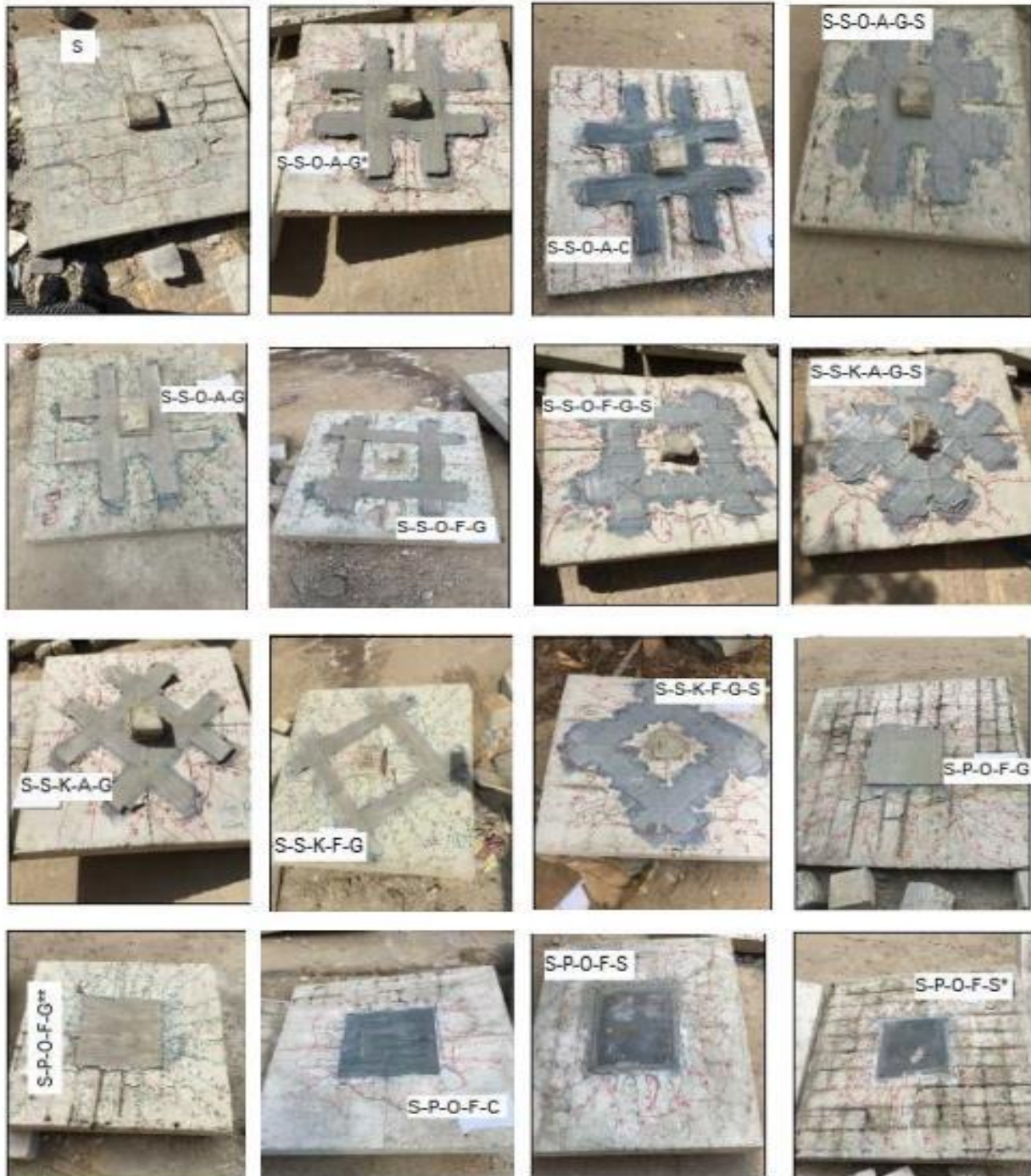
Fig.13. Crack pattern at failure load for the test specimens (bottom faces)
